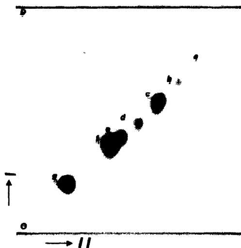
Fig. 8. Separation of partially methylated sugars by two-dimensional t.l.c. Methylated galactose standards were chromatographed in two directions in two different solvent systems. Solvent I : acetone–5% \text{NH}_4\text{OH} (50:1). Solvent II : acetone–28% \text{NH}_4\text{OH} –water (50:5:1). The spots were detected by spraying with the diphenylamine reagent and heating the plate for 1 h at 110^\circ : (a) 2,3,4,6-tetra- O -Me-Gal, (b) 2,3,6-tri- O -Me-Gal, (c) 2,4,6-tri- O -Me-Gal, (e) 2,3,4-tri- O -Me-Gal, (f) 3,4,6-tri- O -Me-Gal, and (g) 2,3-di- O -Me-Gal.
